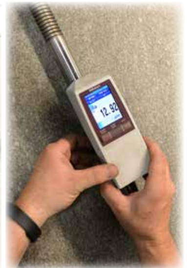
We use an X-ray fluorescence (XRF) analyzer for spot screening of metals (shown at left), and a precision industry standard profilometer is used to measure and verify surface finish.
