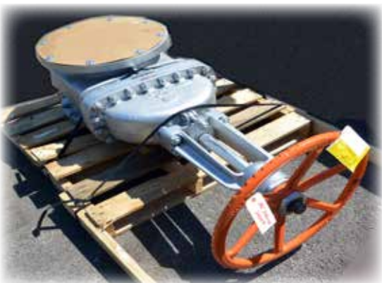
Another gate valve repair is completed: repainted, skidded, and ready to ship.
