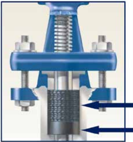
Above: cross section diagram shows location of packing in valve mechanical design. Below: Chesterton packing materials including 1622 low emissions graphite tape are specified for highest reliability.
