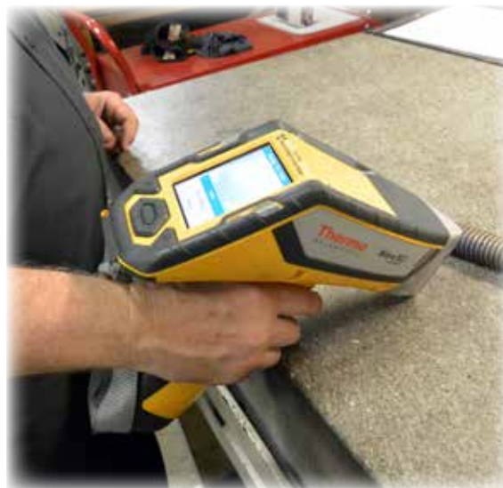
We use an X-ray fluorescence (XRF) analyzer for spot screening of metals (shown at left), and a precision industry standard profilometer is used to measure and verify surface finish.
