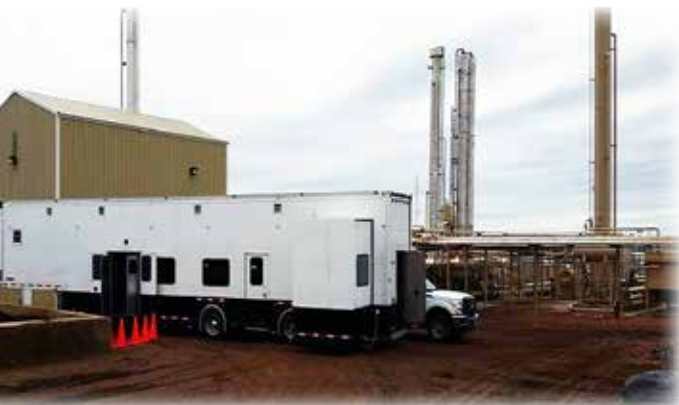
On a typical site visit to a gas processing plant, mobile valve shop technicians perform certified testing and repair services on a full range of pressure relief valves.
